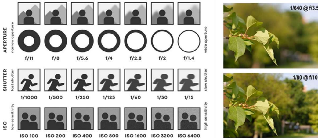
Left: A diagram to show the effect of ISO/ aperture/ shutter speed on focus Right: Two photos showing the effect of aperture on depth of field
